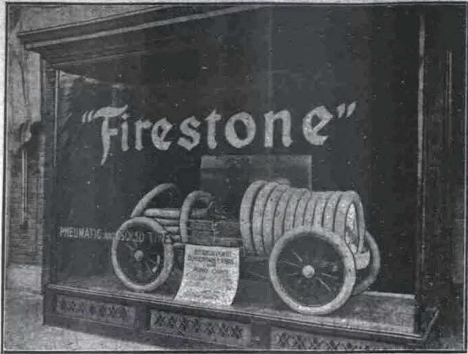
"Roadster" constructed with wood frame, Firestone tires, and the new Firestone special wheels with demountable rims for Ford cars.
