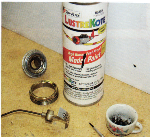
I used the same model airplane paint recommended to repaint your carburetor.
